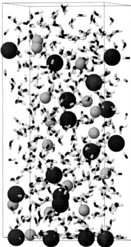
Fig. 25. Snapshot of the simulation with surface charge \sigma = +9.9 \mu\text{C cm}^{-2} . \text{Na}^+ : small spheres, \text{Cl}^- : large spheres. The liquid slab is confined by the metal surface (bottom) and by a 'free' surface (top).
